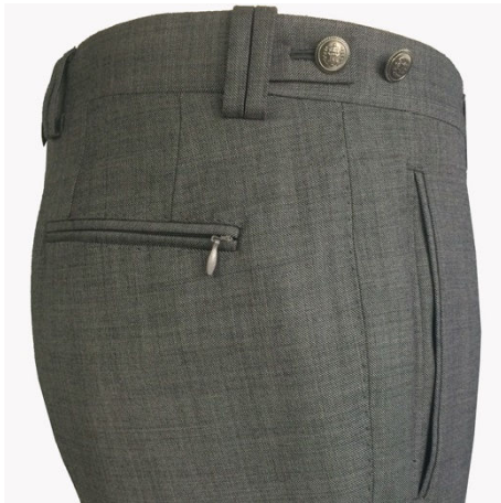
3205 back pockets with zipper 33H0 0.15cm pic stitching around hip pocket
